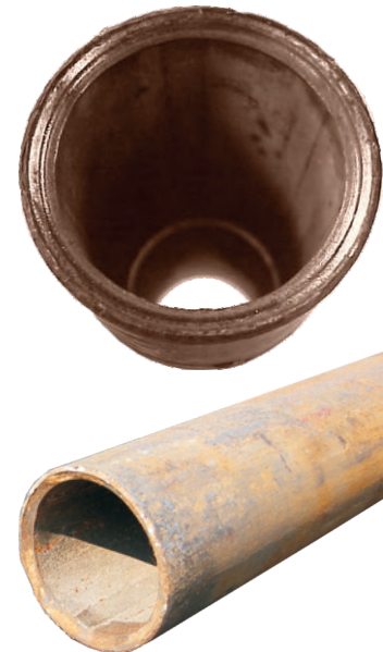
Cuts made with the MCT are superior in smoothness to cuts made with chemicals or a radial cutting torch.
